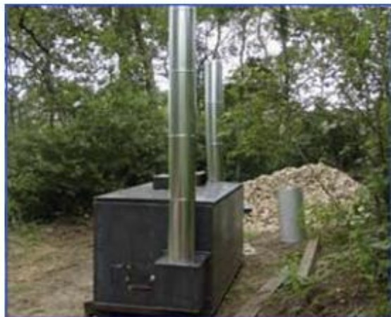
FIGURE 14. RETORT (AN IMPROVED STEEL KILN).
