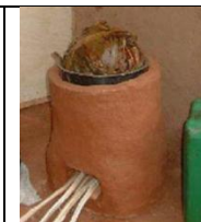
131 Lorena 1 Rocket stove with high insulation
