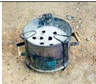
211 Charcoal stove, Old ICS Opening for air may be closed
