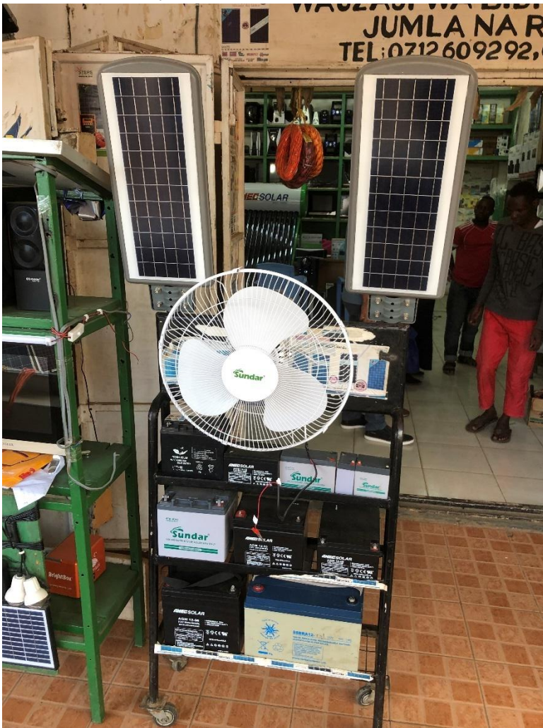
Solar panels and batteries for solar home systems.
