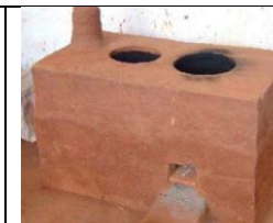
141 Lorena 2 Rocket stove with well- sealed chimney
